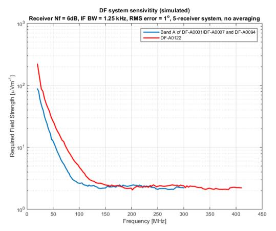
The graph illustrates the direction finding sensitivity of a typical system measured under specific electrical conditions.
